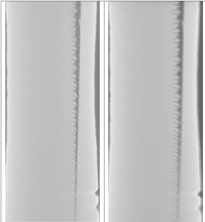
Figure 8. XCT binning and power settings effect on defect detail. The image on the left looks clearer, but does not contain the same blur because the binning has balanced out the curvature on this sample.
