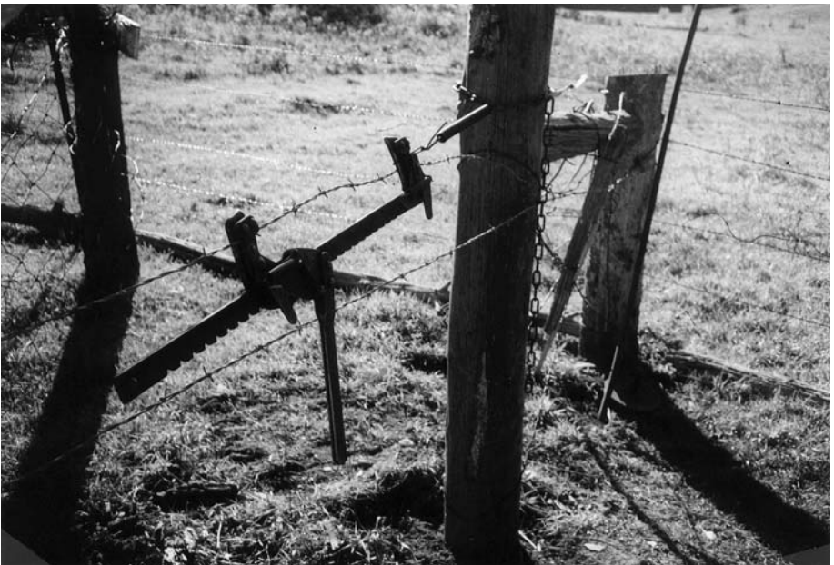
Figure 3. Photograph of end post B showing fence stretcher and spring.
