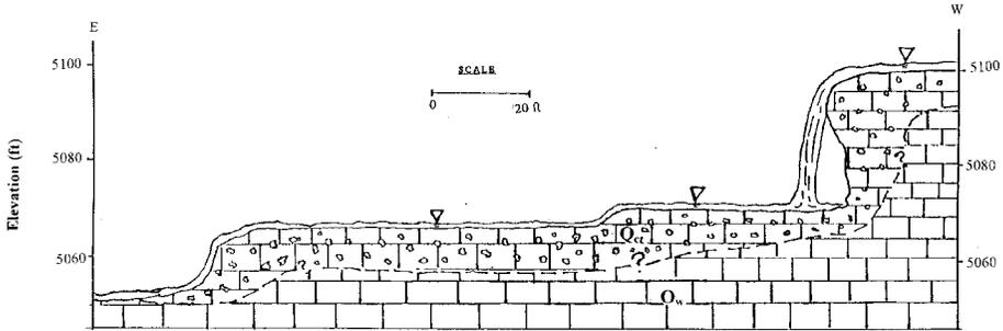
Figure 12. Geologic cross section of Roughlock Falls. Q<sub>ct</sub> is the calc-tufa, O<sub>w</sub> is the Whitewood Dolomite.
