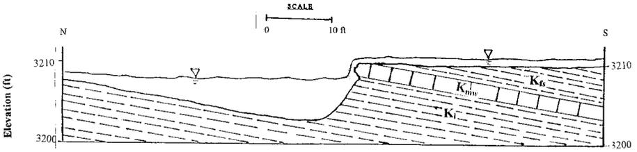
Figure 8. Geologic cross section of Cheyenne River falls.  $K_{fs}$  is the Fuson Shale,  $K_{ms}$  is the Minnewasta Limestone, and  $K_i$  is the Lakota formation.
