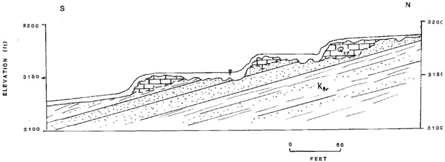
Figure 10. Geologic cross section of the Fall River falls.  $Q_{ct}$  is the calc-tufa,  $K_{fr}$  is the Fall River Formation.
