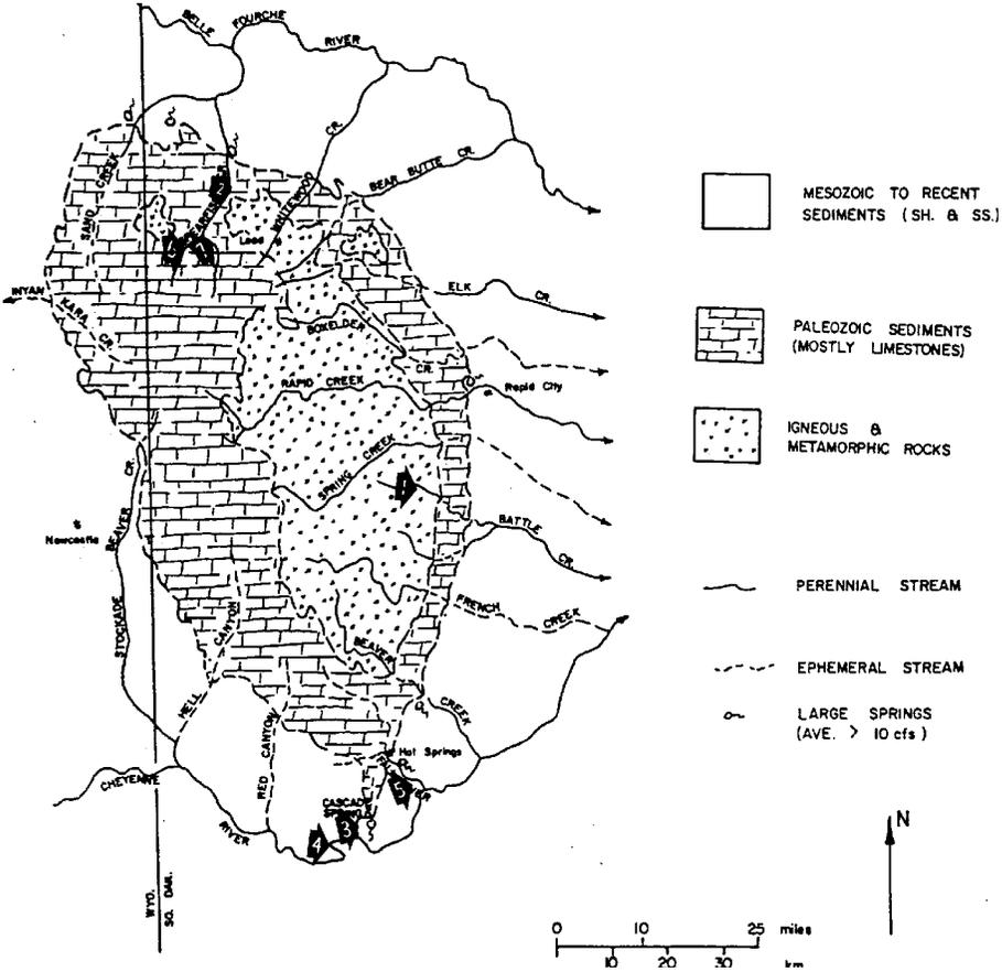
Figure 1. Generalized geologic map of the Black Hills and its relationship to stream flow, showing the location of waterfalls (map taken from Rahn et al, 1981). Numbers 1 to 7 refer to waterfalls shown in Table 1.
