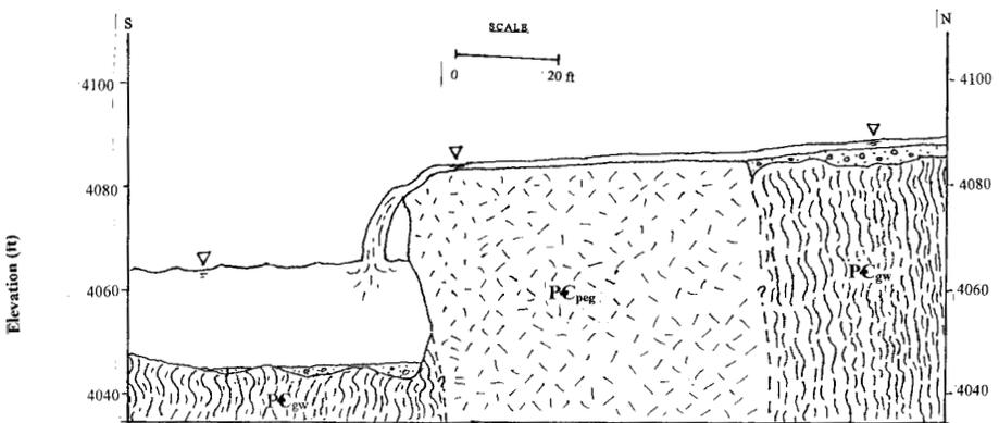
Figure 2. Geologic cross-section of Big Falls on Battle Creek. PC<sub>peg</sub> is the pegmatite, PC<sub>gw</sub> is the Metagraywacke.
