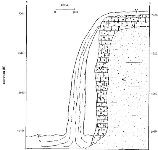
Figure 14. Geologic cross section of Spearfish Falls.  $Q_{ct}$  is the calc-tufa,  $C_d$  is the Deadwood Formation.
