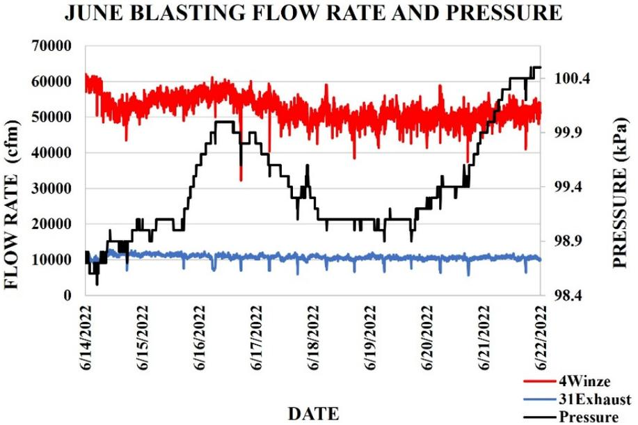
**Figure 16. Nine Ledge Four Winze Wye Pressure and flow rates 7 days in June 2022. Pressure and flow rate spike signature of blast door closure. The flow rate in June is higher than in October. The red and blue lines are flow rates plotted to the left axis and the black line is pressure plotted to the right axis.**
