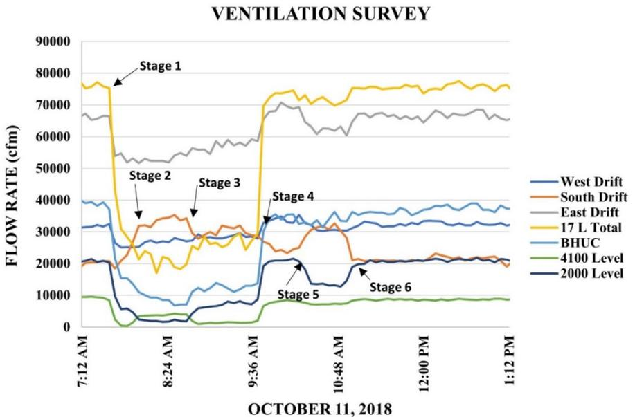
**Figure 4. Ventilation survey showing the response of the flow meter network during the six stages of fan configuration testing.**
