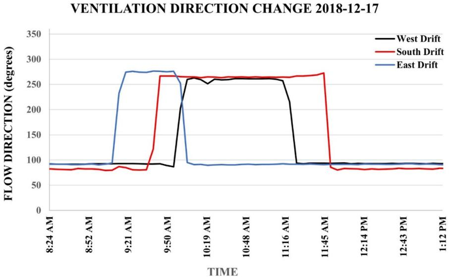
Figure 22. Data from one ventilation direction change in each of the three drifts in the science triangle. The West drift is plotted in black, the South drift in red and the East drift in blue.
