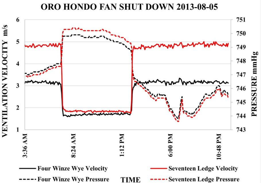
Figure 3. During a ventilation fan outage event, air velocity decreases and air pressure increases at two locations on the 4850L. Air velocities are plotted on the left axis with solid lines and the air pressure is plotted on the right axis with dotted lines.
