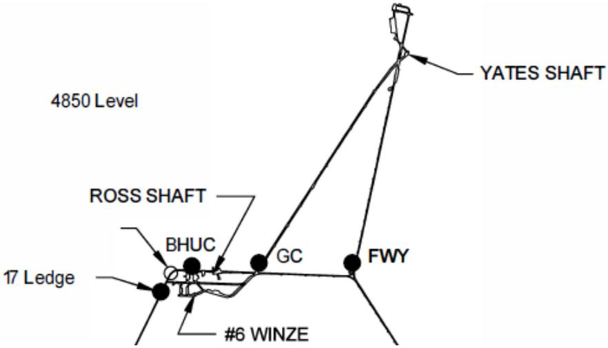
Figure 2. Location of flow meters in the 4850L.
