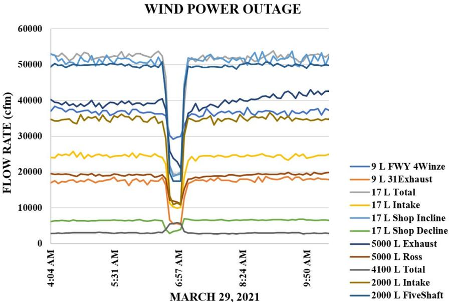
**Figure 6. A power outage on March 29, 2021, affected every level with a flow meter station.**
