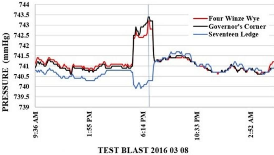
Figure 11. The pressures increased at the Four Winze Wye and Governor's Corner and decreased at Seventeen Ledge because the ventilation changes were made to exhaust the gases out of Four Winze Wye.
