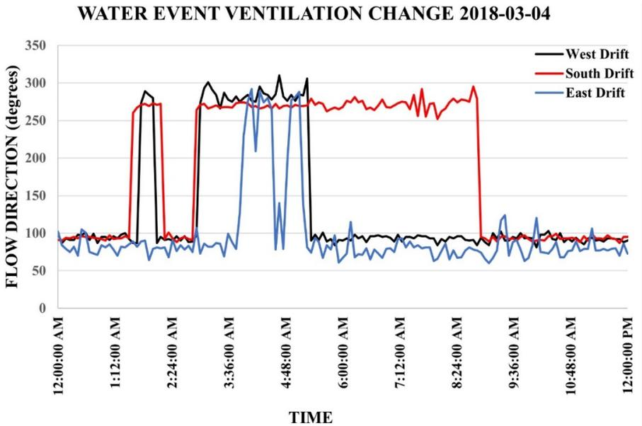
Figure 21. Two different ventilation direction changes for each of the three drifts in the science triangle at the 4850L. The West drift is plotted in black, the South drift in red and the East drift in blue.
