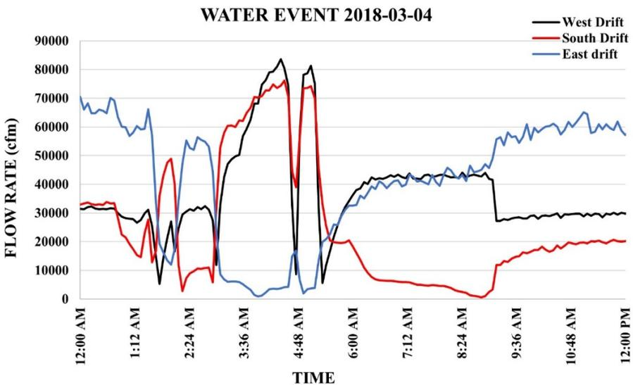
**Figure 19. Water event in March of 2018 showing flow rate changes in the science triangle at the 4850L. The West drift is plotted in black, the South drift in red and the East drift in blue.**
