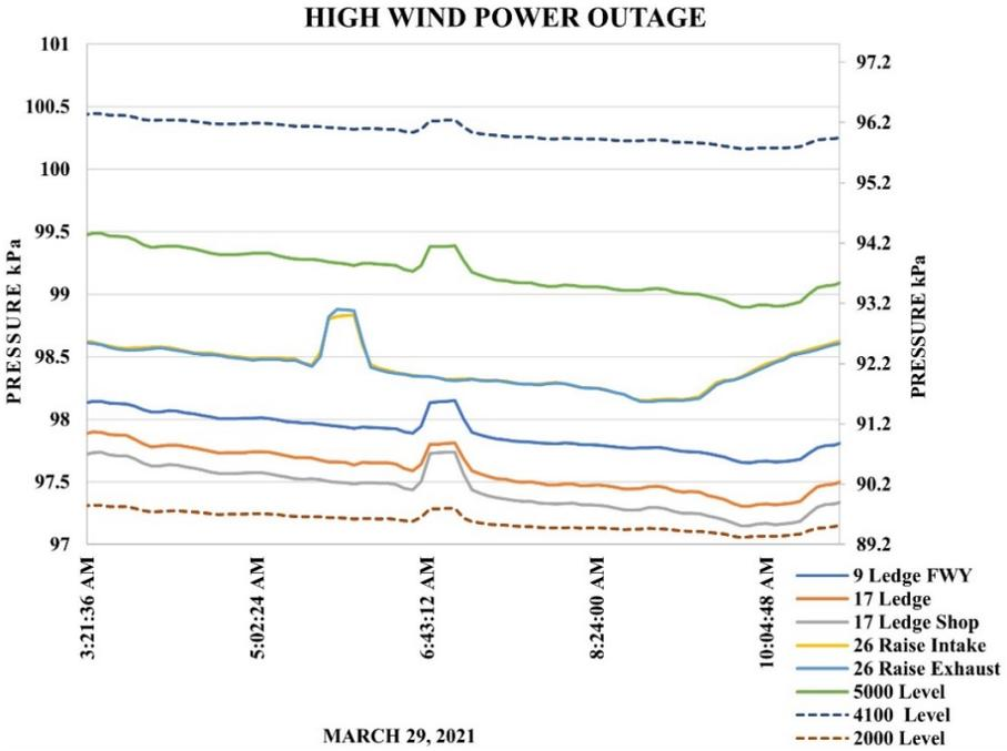
**Figure 5. Underground air pressure changes measured during a power outage at SURF. The 2000L and 4100L flow meters with the dotted lines are plotted to the right axis. The nine ledge, 17 ledge, 26 Raise and the 5000L flow meters have solid lines and are plotted on the left axis.**
