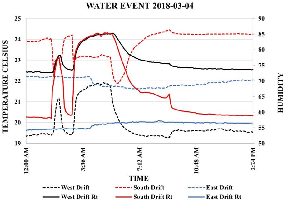
Figure 23. Water events showing data signatures that have larger effects in temperature and humidity. The dotted lined temperatures are plotted to the left axis with the West drift in black the South drift in red and the East drift in blue. The humidity levels are the solid lines plotted to the right axis with the West drift in black the South drift in red and the East drift in blue.
