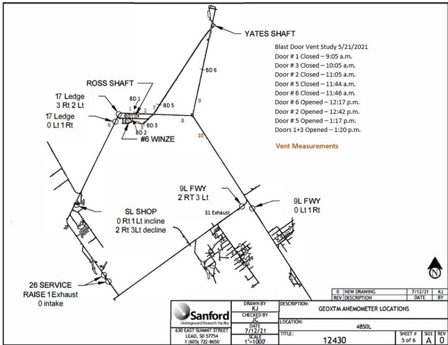
Figure 13. The full 4850L SURF showing locations of the flow meters on that level.
