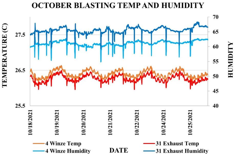
**Figure 17. Nine Ledge Four Winze Wye Temperature and Humidity for 7 days in October 2021. Temperature and Humidity changes though small are detectable. The temperatures in orange and red are plotted to the left axis and the blue humidity lines are plotted to the right axis.**
