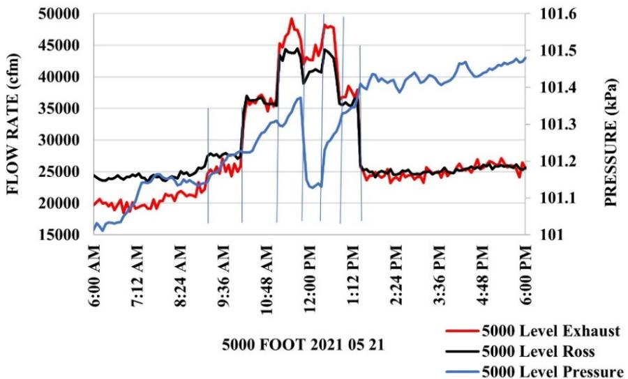
Figure 14. All phases of the blast door closure shown at the 5000L. Air flow with the red and black lines are plotted to the left axis and pressure in blue is plotted to the right axis.
