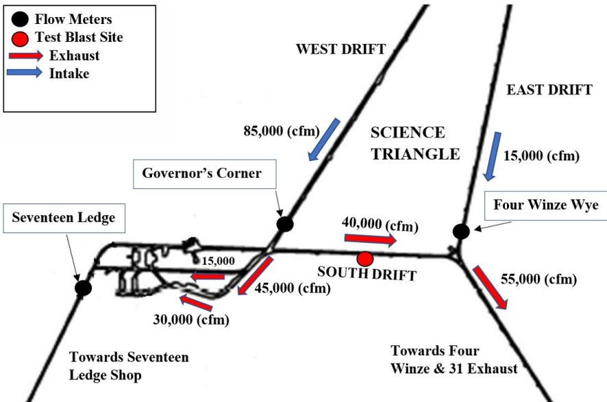
**Figure 8. LBNF Blast Vibration Study-SDSTA Blast Plan, December 4, 2015 (Vardiman 2015). This design is to exhaust blast gasses out towards Four Winze and 31 Exhaust. The black dots show the flow meter locations, and the red dot shows the test blast location.**
