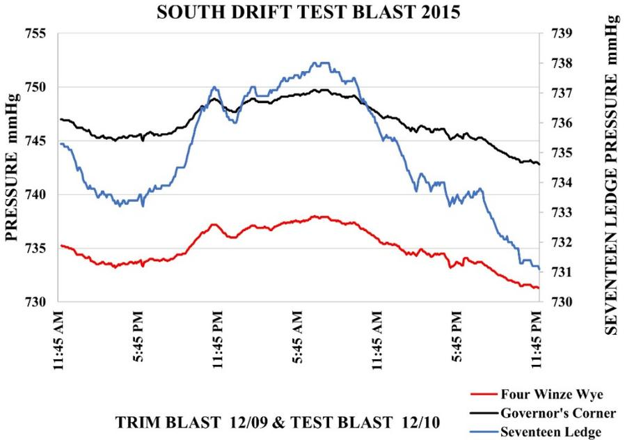
**Figure 9.** Pressure wave of trim blast detected by the three flow meters on the 4850L Seventeen Ledge flow meter is plotted to the right because it was not calibrated with the other two flow meters.
