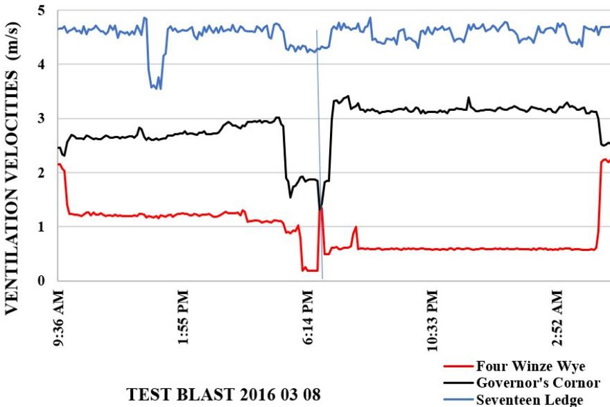
Figure 12. Air velocity recorded at Governor's Corner (West Drift) and Four Winze Wye (East Drift) decreased prior to blast. After the blast Governor's Corner (West Drift) increased to expel exhaust gases down Four Winze Wye drift.
