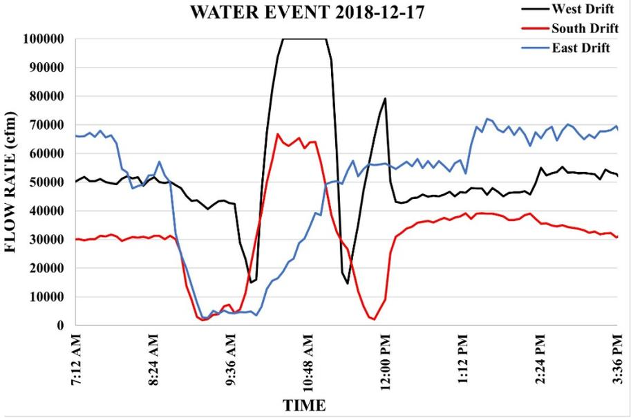
Figure 20. Water event in December of 2018 showing flow rate changes in the science triangle at the 4850L. The West drift is plotted in black, the South drift in red and the East drift in blue.
