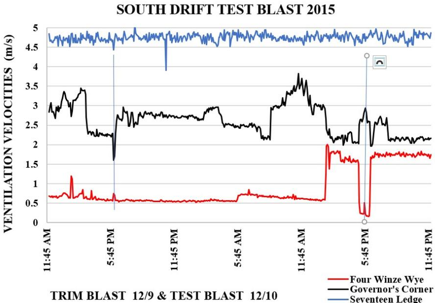
**Figure 10.** The ventilation changes for the trim and test blasts. The trim blast occurred at 6:00 p.m. on the 9<sup>th</sup> and the test blast occurred at 6:00 p.m. on the 10<sup>th</sup>.
