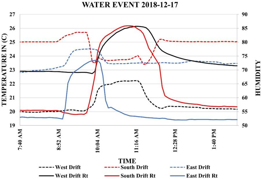
**Figure 24. The December water event showing a data signature that having larger effects in temperature and humidity. The dotted lined temperatures are plotted to the left axis with the West drift in black the South drift in red and the East drift in blue. The humidity levels are the solid lines plotted to the right axis with the West drift in black the South drift in red and the East drift in blue.**
