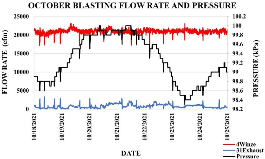
**Figure 15. Nine Ledge Four Winze Wye Pressure and flow rates for 7 days in October 2021. Pressure and flow rate spike signature of blast door closure. The red and blue lines are flow rates plotted to the left axis and the black line is pressure plotted to the right axis.**
