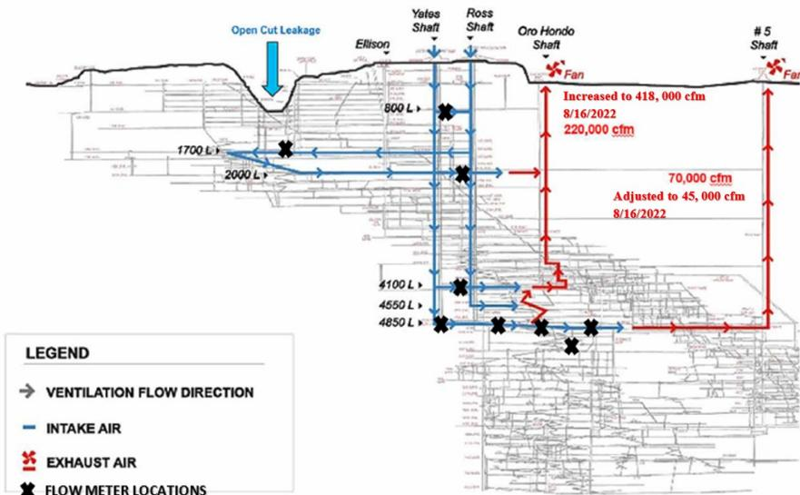
Figure 1. SURF ventilation model with flow meter locations (Artz et al. 2015).
