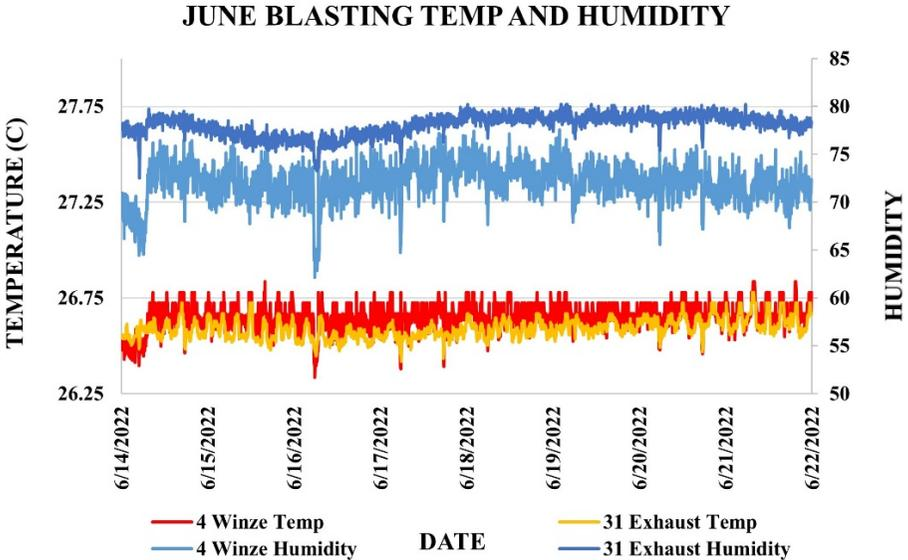
**Figure 18. Nine Ledge Four Winze Wye Temperature and Humidity for 7 days in June 2022. Temperature and Humidity changes are harder to distinguish. The temperatures in orange and red are plotted to the left axis and the blue humidity lines are plotted to the right axis.**
